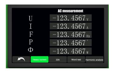
Click "Heavy current" or "10A" to select corresponding gear while "Heavy current" can be used in direct perforation measurement, "10A" can be used when accessing 10A small current.
